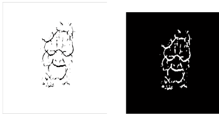
Figure.5. Result of the image morphology process showing the top-hat segmented image and its complement image.
