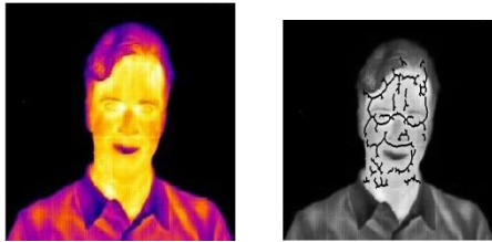
Figure. 8 Illustrative of thermal template overlaid on the thermal image of the subject.
